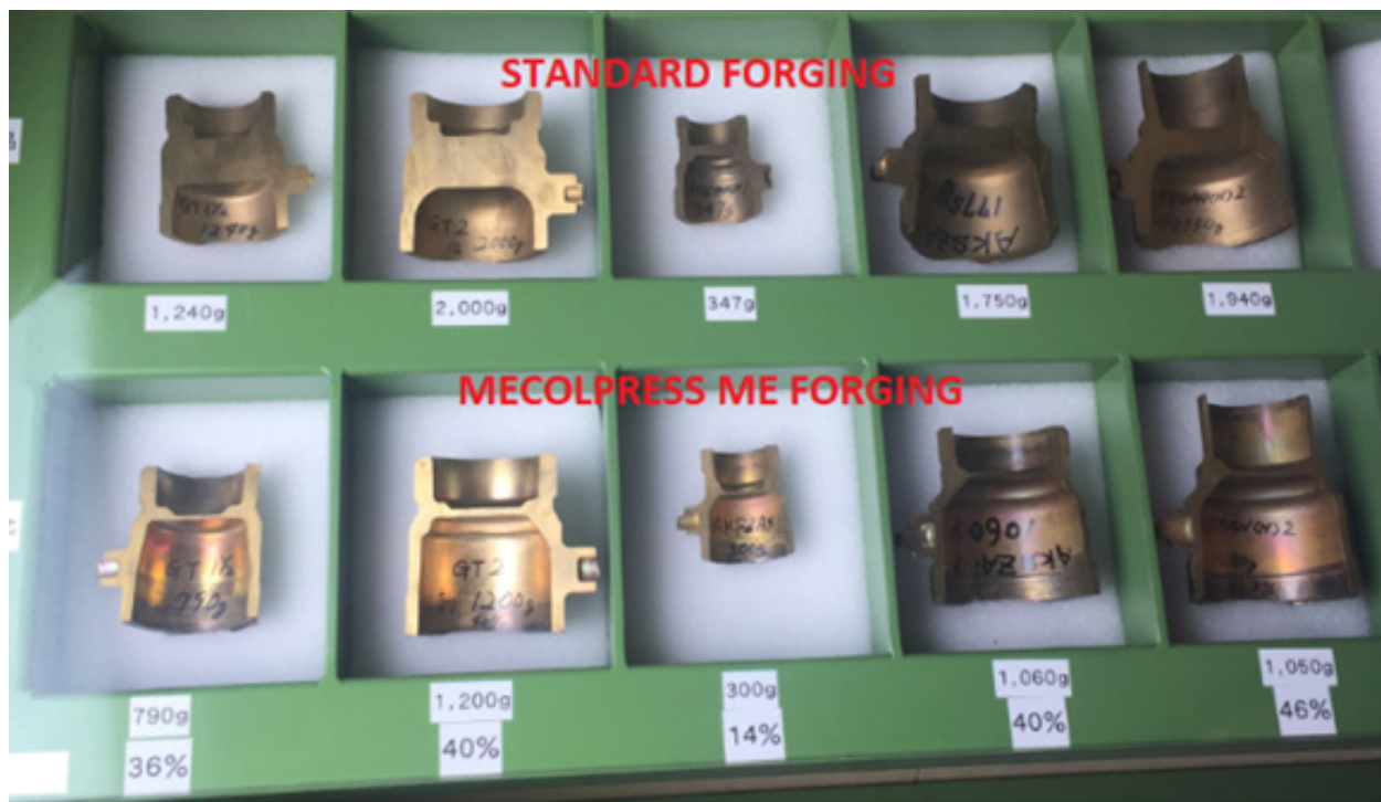
Mecolpress ME Next Generation series hydraulic press outstanding parts weight reduction
