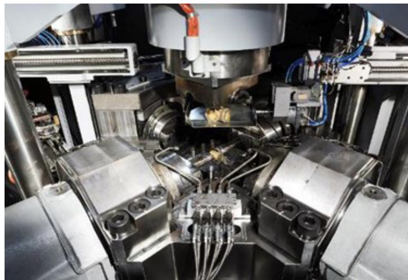
Mecolpress ME Next Generation series hydraulic press hot forging EG coring tool
